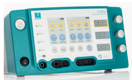
Fig. 4: CURIS® 4 MHz radiofrequency generator.
