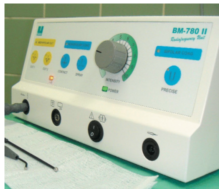
Figure 1: Radiofrequency unit (RF generator) BM-780 II with 2 mm straight and 3 mm angled ball electrodes
