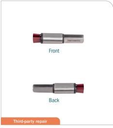
The connector of the CE-marked instrument has been replaced. The labeling indicates the mandatory batch number and CE marking according to article 20 of the regulation (EU) 2017/745 (MDR).
