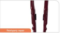
The patented Guide-Stop™ has been modified. This may change the spring force of the forceps and the tips may not close precisely.
