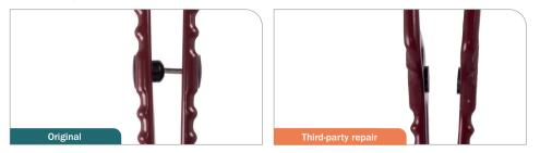
The patented Guide-Stop<sup>™</sup> has been modified. This may change the spring force of the forceps and the tips may not close precisely.
