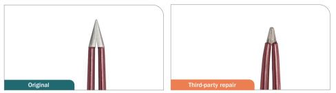
The tips have been repaired, which significantly changes the characteristics of the forceps and may affect the performance.
